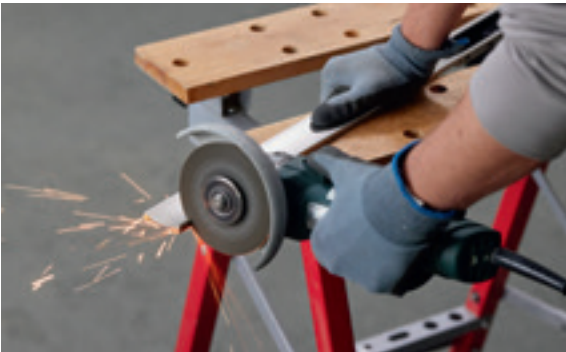
↑ Profiles can be cut to length to suit different requirements.
